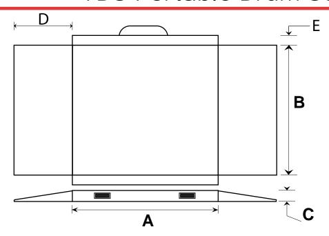
TDS platform is made out of industrial weight heavy duty 1/4" checkered thread steel plate baked powder painted. Two built in folding ramps are low enough to get the hand truck on with ease. Lifting handle and built in wheels for easy moving. Platform uses standard (4) 3 mv/v, 350 ohm load cells and stainless steel signal trim summing junction box. For easy leveling, top bubble level is included. Live rail makes the weighing surface even larger than 36". Adjustable height from 2" to 4.5"
